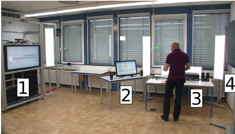
Figure 4.4: The figure shows the setting in which we have tested our assistant. The home entertainment system can be seen on the right side: (3) shows the user interacting with the blu-ray player, satellite receiver, and amplifier. On its right side, (4) shows the television. The assistant runs on separate devices. (1) shows the main interaction device, which is a large touch screen that also features input via pointing gestures (for which it is equipped with a set of cameras) and speech input. (2) is an additional device that also features input via touch and speech. On the right side of the main interaction device, we can see one of two laser-range-finders for localization of the user. (The picture is an edited version of a screenshot taken from a video describing our system [A22]; see http://companion.informatik.uni-ulm.de/ie2014/companion-system.mp4 at approx. 18:46/20:26.)
